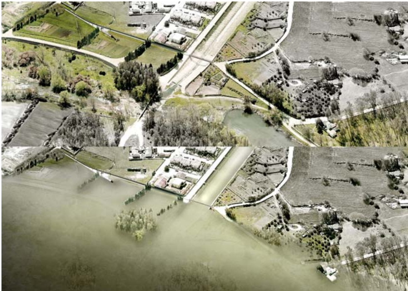
Fig. 3 Aerial view in normal conditions and during a 50 years return period
